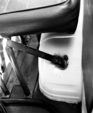
PANEL-BEATEN: The seat in this Quantum panel van has been welded to the floor, instead of the chassis, to turn it into a taxi. Picture: KATHERINE MUICK-MERE
